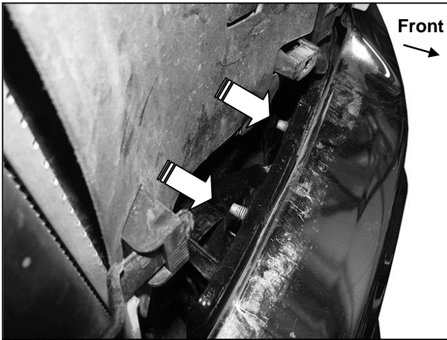
(Fig 3) Remove driver side top bumper hardware
