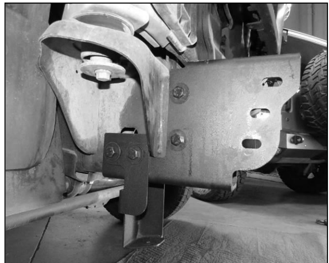
(Fig 9b) Skid plate bracket sandwiching the mounting bracket and frame.
