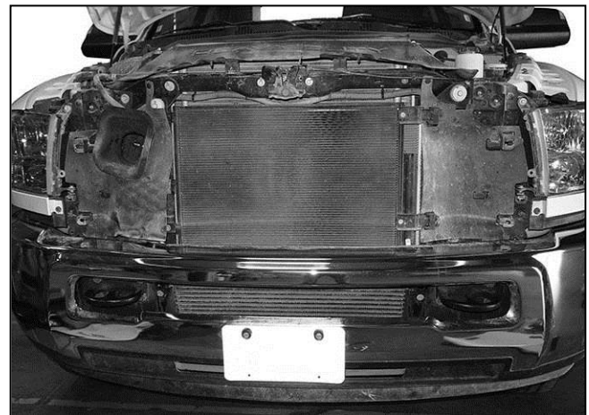
(Fig 2) Remove radiator top cover and grille
