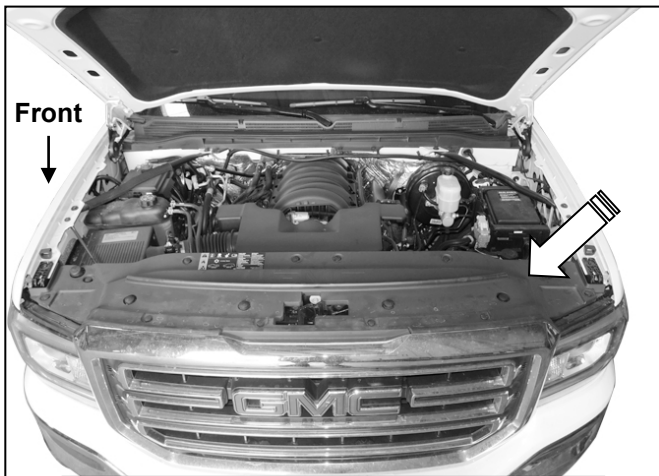
(Fig 5) Remove the plastic cover (arrow)
