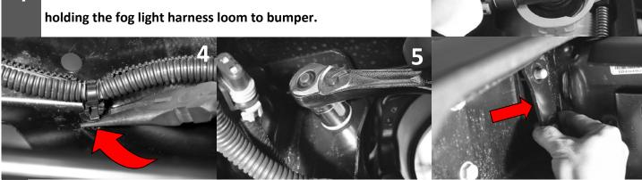
5 Remove the nuts holding the factory bumper on, four (4) on each side using an 18mm socket and socket wrench. Keep the backing plate for installing Road Armor Bumper.
