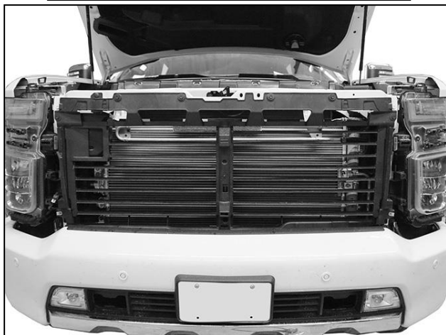
(Fig 7) Grille and fascia removed
