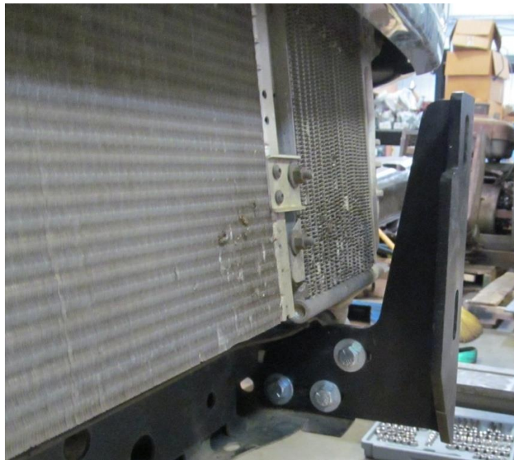
FIGURE 9: INSIDE VIEW OF FRAME MOUNTS
