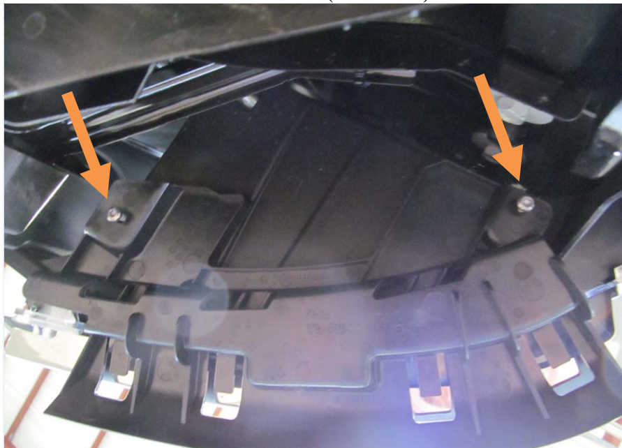
16. Remove two screws holding on plastic trim under headlight with T15 Torx bit. Set bracket aside. (both sides)
