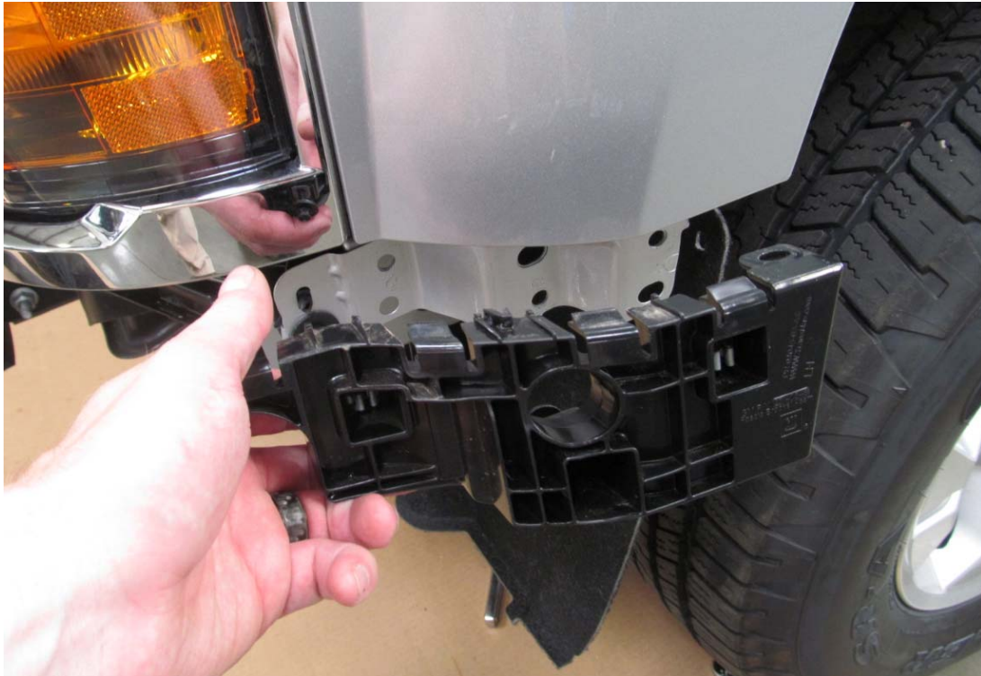
16. Remove two screws holding on plastic trim under headlight with T15 Torx bit. Set bracket aside. (both sides)
