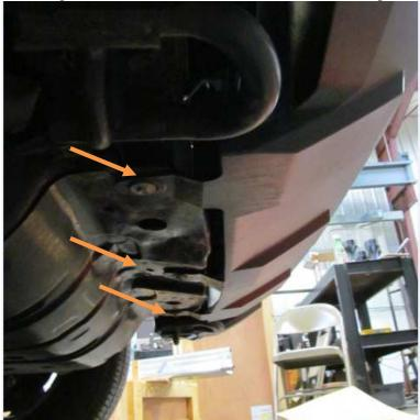
3. Using 17mm socket, Remove two bolts holding on OEM tow hooks. (both sides)
