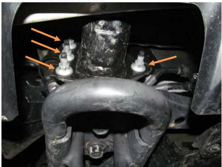
5. Pull bumper forward off of studs and move down so inner fenders will clear frame.
