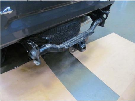
17. Install bolt closest to cab that was removed and tighten.
