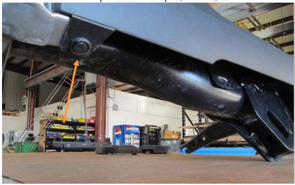
10. Using Phillips head screwdriver, remove plastic screw in middle of bumper where license plate was. Then remove remainder of clip.
