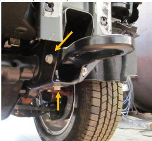
9. Remove OEM wiring harness, sensors and outer grommets from OEM bumper. (if applicable) When removing sensors and grommets, keep them in the same order and orientation left to right that they came out of the truck in. This is very important. Use pic below to keep track of sensors and grommets.
