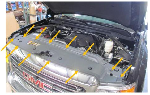
2. Using 10mm socket, remove four screws in top of grill.
