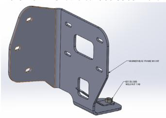
8. Install Hammerhead bumper on frame mounts using bolts, flat washers, lock washers, and nuts from Hardware Kit#1 and ¾" wrench and socket.
