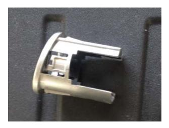
2. Install Hammerhead sensor grommets in two center holes of Hammerhead bumper. Then install OEM sensors and wiring harness. Make sure the sensors are oriented in the same way they were in the OEM bumper.
