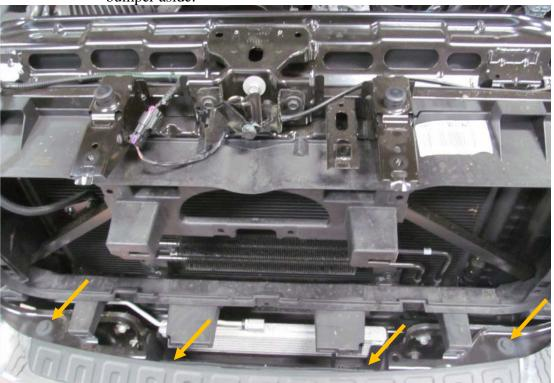
7. Using 15mm socket, remove eight bolts holding on OEM bumper brackets. Set brackets aside.
