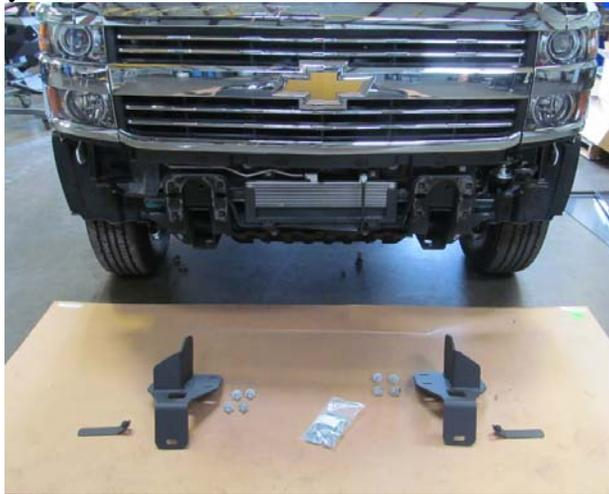
6. Using OEM hardware, install Hammerhead Frame mounts on frame as shown. Do not fully tighten.
