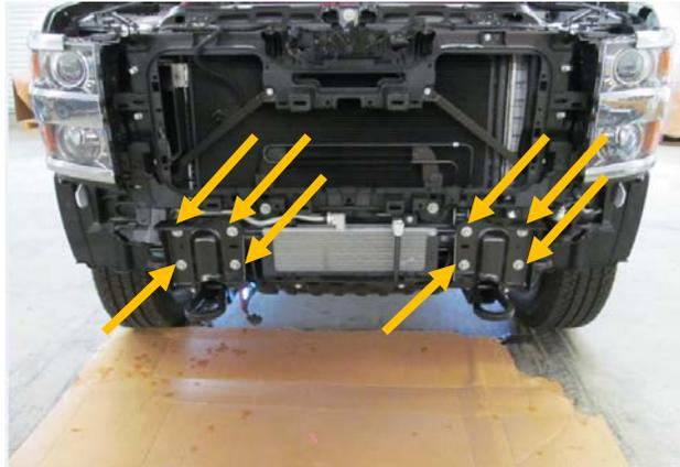
8. Using 18mm socket and wrench, remove OEM tow hook. Set tow hook aside. (both sides)
