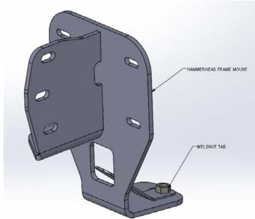
8. Using hardware from kit #62 and weldnut tab 3 (qty-2), install Hammerhead bumper on frame mounts. Run bolts toward the center of the vehicle and use weldnut tab 3 on inside. This will make the bolts easier to reach with wrench or socket when tightening.
