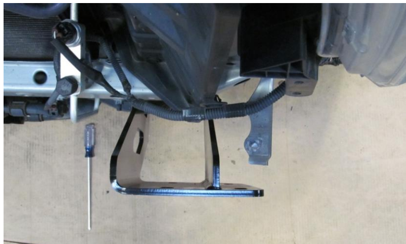
Figure 20: TOP VIEW OF DRIVER SIDE FRAME MOUNT
