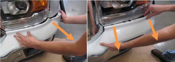
5. Release six tabs on center of plastic trim below the grill. Have a friend gently pull out on the plastic trim as you release the tabs behind the
