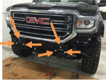
11. Remove two bolts attaching OE tow hooks with 18mm socket and wrench. (both sides) Set tow hooks aside.
