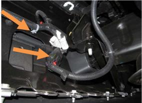
7. Remove OE bumper bolt behind bumper with 18mm socket. (both sides)
