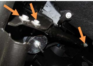
9. Remove OE bumper bolt with 18mm wrench. (both sides) Remove OE bumper and set aside.
