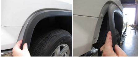
3. Remove screw holding on plastic trim piece with 7mm socket. (both sides)
