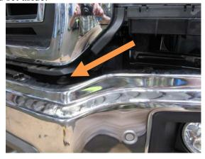
10. Remove six bolts holding on OE frame flanges to frame with 15mm socket.
