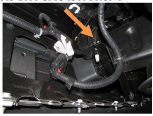
8. Remove three bolts from OE side bumper support (in front of tires) with 15mm socket. (both sides)
