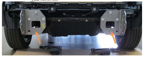
3. Install Hammerhead lower frame mounts (601-56-2155 and 601-56-2156) and loosely tighten. Use OE hardware for thru frame bolt and use two ½"-13 x 2" bolts, four flat washers, two lock washers and two nuts from Hardware kit #1 for the lower bolts. (orange arrows).
