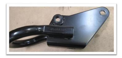
8. Using an 18mm socket, remove two nuts on bolt strip. (Both Sides)
