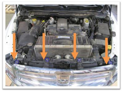
3. Using 18mm socket remove two nuts from the top of the bumper bracket.(Both Sides)
