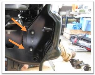
9. Using 13mm socket, <u>LOOSEN</u> bolts from intercooler bracket. <u>DO NOT REMOVE</u>. (Both sides)
