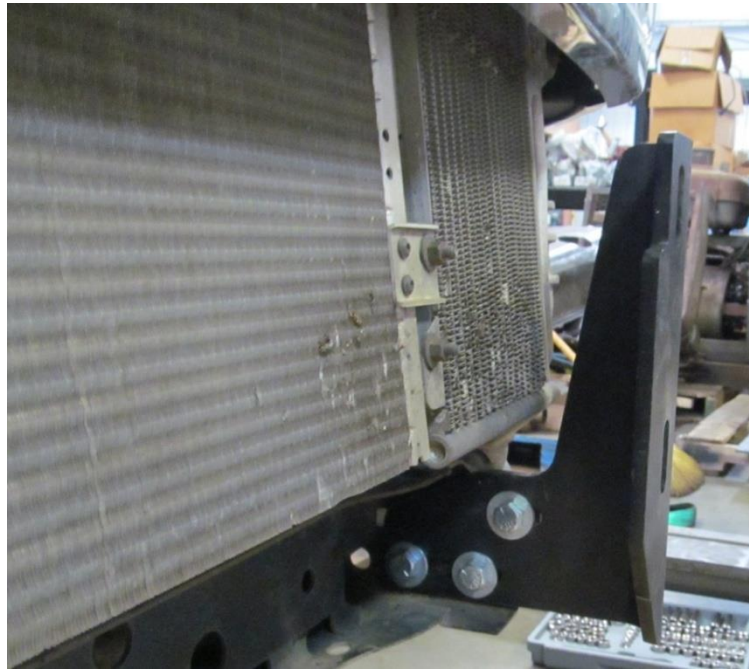
FIGURE 9: INSIDE VIEW OF FRAME MOUNTS
