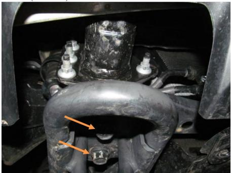
4. Using 14mm socket, Remove four nuts holding on OEM bumper. (both sides) Be careful, the bumper will be ready to come off after these bolts are removed.
