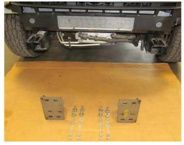
3. Install frame mounts on frame with hardware from kit #98. Insert bolts from the top. Use bolt strips removed in step 5 to attach HH mount on outside of frame. Do not fully tighten.
