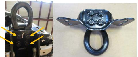
5. Using 18mm socket, remove two nuts attaching underrun bracket to frame. Set aside; it will not be reused. (both sides) Bolt strips and nuts will be reused.
