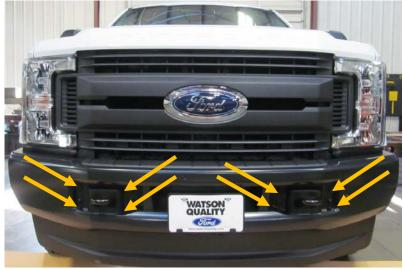
4. Using 18mm socket, remove four bolts attaching tow hook to frame. Set aside; it will not be reused. (both sides)
