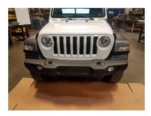
1. Remove 8 plastic clips from front of OE "skid plate". Using the 8mm socket, remove the 2 bolts from the bottom then remove the skid plate.
