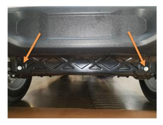
3. There are two 18mm nuts on the outside of the frame and the inside of the frame for a total of 8. Remove these with the 18mm socket.
