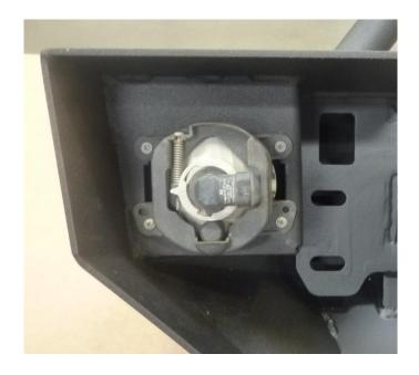
2. Install four  $\frac{1}{2}$ "-13 x 1.5" carriage head bolts in bumper with push nuts. Do this for both sides
