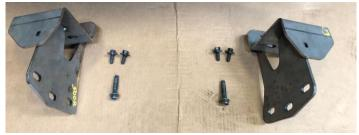
4. Using a 14 mm socket or wrench, a 17 mm socket or wrench, and hardware from hardware kit #188, attach the frame mounts to the frame of the truck. Use 4 washers on each of the bottom mounted OE bolts. Do not fully tighten.
