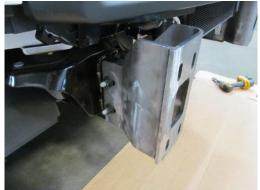
8. Attach Hammerhead bumper to frame mounts using eight ½" -13 bolts, sixteen ½" flat washers, eight ½" lock washers, and eight ½" nuts from Hardware kit 1.
