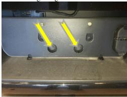
5. Remove the two <u>nuts</u> holding the bumper to the frame on both sides. You will use a 16mm socket.
