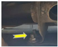
4. Align and level bumper with the truck. Tighten the center bolts with a 15mm socket and bumper mount bolts with a ¾ wrench and socket. Install license plate mounting kit and license plate on bumper.
