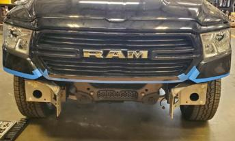
8. Using a hoist or a few friends, attach bumper to frame mounts using hardware kit #58 and weldnut tabs. Start all bolts before aligning bumper. Leave a minimum of 3/8" space between bumper and truck body. When the truck flexes off-road, this distance allows your bumper and truck body to have clearance. Tighten bolts with 3/4" socket and wrench. Tighten frame mount bolts at this time.
