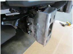
8. Attach Hammerhead bumper to frame mounts using eight <sup>1</sup>/<sub>2</sub>" -13 bolts, sixteen <sup>1</sup>/<sub>2</sub>" flat washers, eight <sup>1</sup>/<sub>2</sub>" lock washers, and eight <sup>1</sup>/<sub>2</sub>" nuts from Hardware kit 1.
