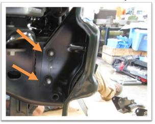
9. Using 13mm socket, <u>LOOSEN</u> bolts from intercooler bracket. <u>DO NOT</u> <u>REMOVE</u>. (Both sides)
