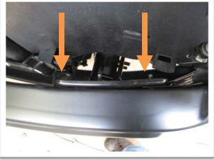
4. Using 18mm socket remove two nuts holding on bottom of bumper bracket to bumper. (Both sides)
