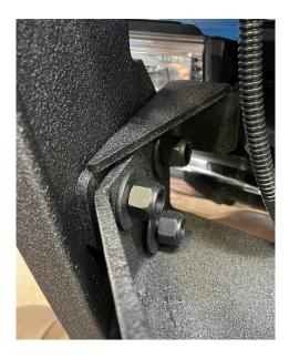
5. Following steps outlined in Defender Series grille guard install instructions, fully tighten all hardware using ¾" socket. Install winch into winch tray using hardware supplied by winch manufacturer at this time.
