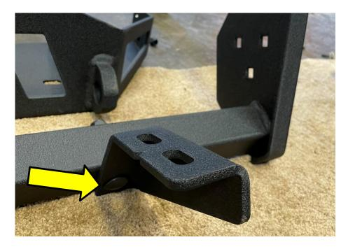
2. Slide the grille guard into place from the back of the grille guard as shown below. Using (2) 1.5" carriage head bolts, (2) flat washers, and (2) nylock nuts supplied in hardware kit #216, fasten winch tray to the grille guard on either side of the winch tray using the lowest mounting points in the grille guard uprights as shown below. Do not fully tighten.
