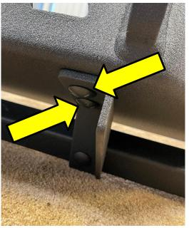
4. Using install instructions provided with your defender series grille guard, install grille guard onto truck at this time. When mounting lower frame mounts to grille guard, be sure to slide frame mounts in between grille guard upright and winch tray as shown below.
