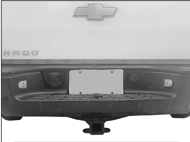
(Fig 1) Remove license plate and spare tire access lock. Unplug and remove license plate lights, and trailer plug if equipped
