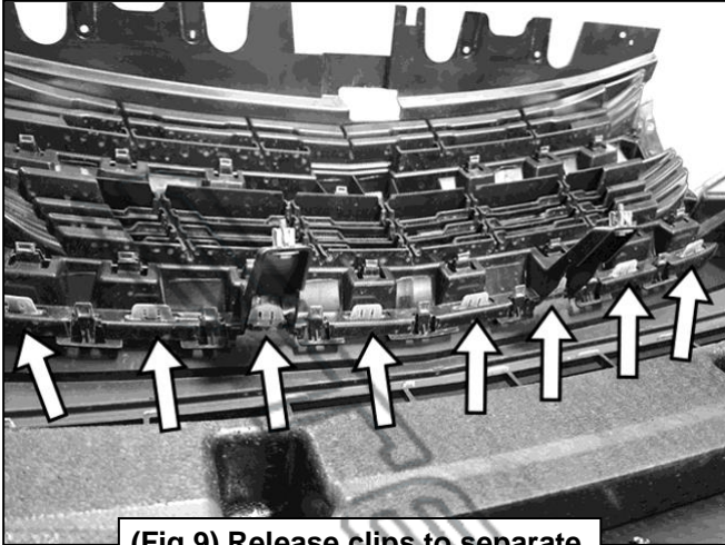
(Fig 9) Release clips to separate grille from bumper (arrows)
