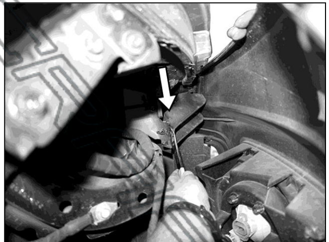
(Fig 8) Pull back loose end of bumper cover to locate inner attachment location for grille below headlight. Use a flat blade screwdriver to carefully pry clips out from bracket to release grille and bumper cover (arrow-passenger/right location pictured)
