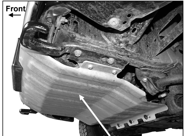
(Fig 4) Remove skid plate if equipped
