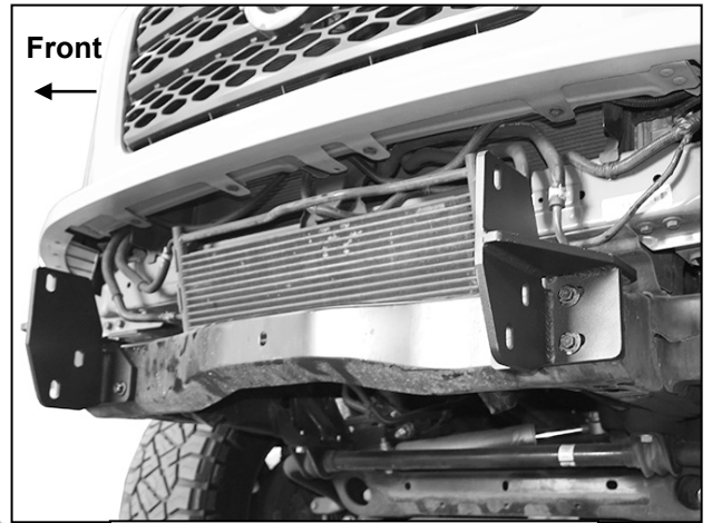
(Fig 9) Frame Brackets installed
