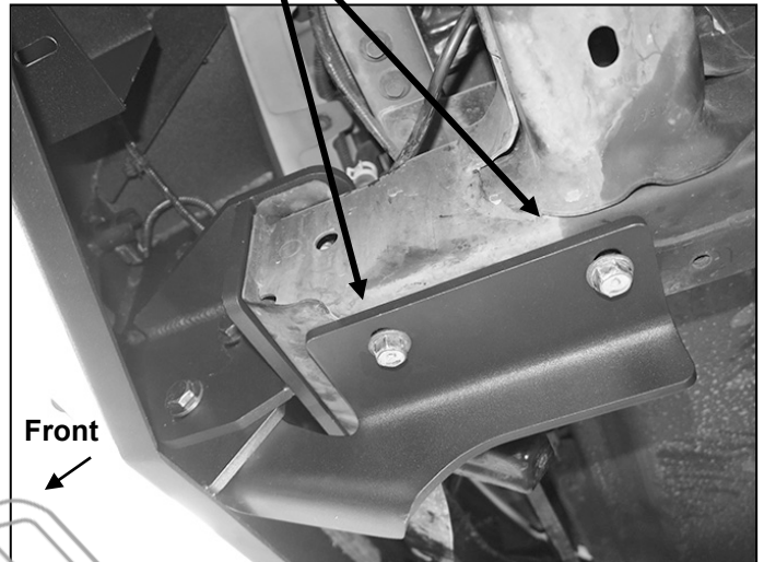
(Fig 19B) Attach Support Bracket to bottom of frame, (driver/left side pictured from behind bumper)
