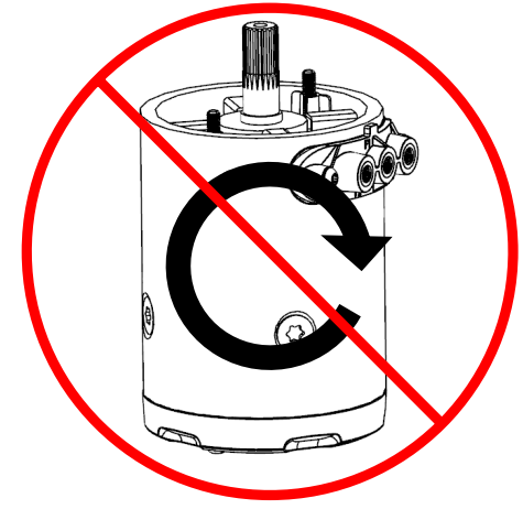
6 Do NOT hold or place motor with shaft UP. The motor may disassemble.
