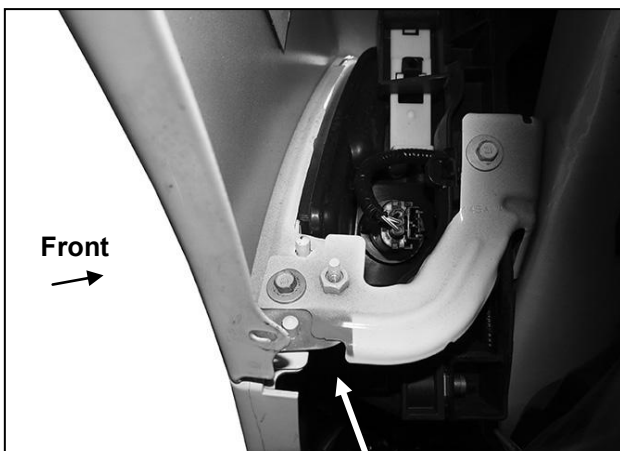
(Fig 3) Pull back fender liner to locate fascia attachment at bottom of front fender
