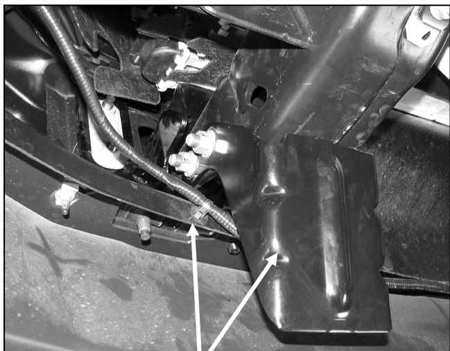
(Fig 1) Driver side lower frame extension and fog light wire harness pictured from behind bumper
