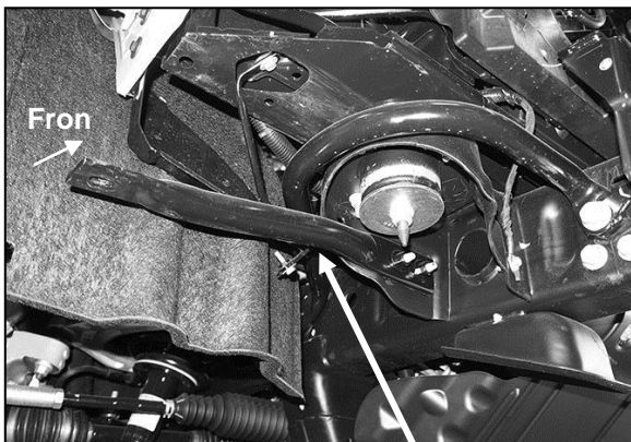
(Fig 4) Remove outer bumper support brackets
