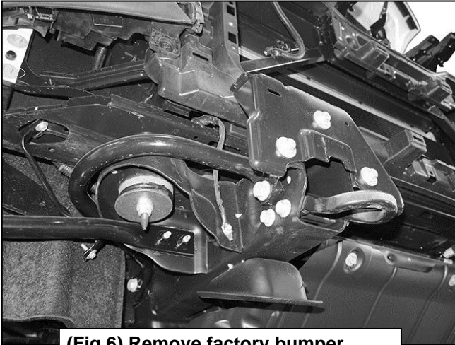
(Fig 6) Remove factory bumper brackets and tow hooks if equipped
