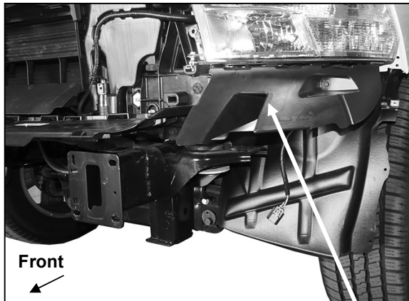
(Fig 6) Remove plastic block from below headlight
