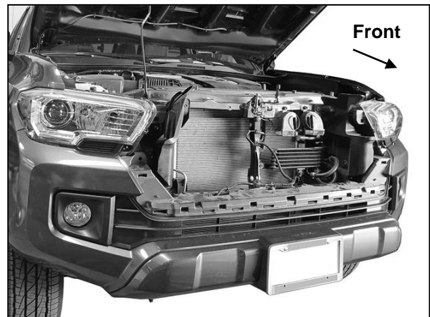
(Fig 2) Remove grille, air dam from below bumper and license plate. Remove plastic bumper cover
