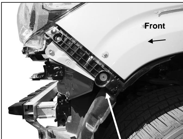
(Fig 3) Remove plastic block from front edge of fender. NOTE: Reinstall hardware to secure headlight. Reinstall grille and cover
