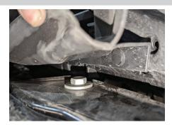
Remove the 10mm bolts from the lower bumper.
