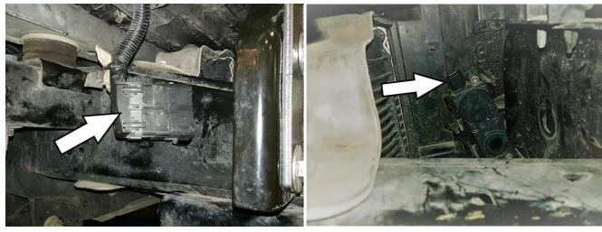
2. To remove the factory bumper, you will need to remove the six 21mm mounting nuts (three on each frame horn). There will be one more connector above the bottom louver system on the driver side. Carefully pull the bumper away from the frame then unplug connector.
