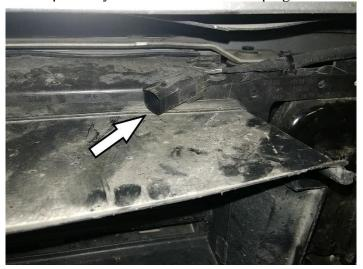
3. If tow hooks are present, remove them. Mount the bottom brackets along with the tow hooks to the bottom of the frame. Mount the top brackets to the two outside holes in the frame plate. Use ½" hardware provided. Brackets should be about 39 ½" O.D. apart. (Hand tighten)
