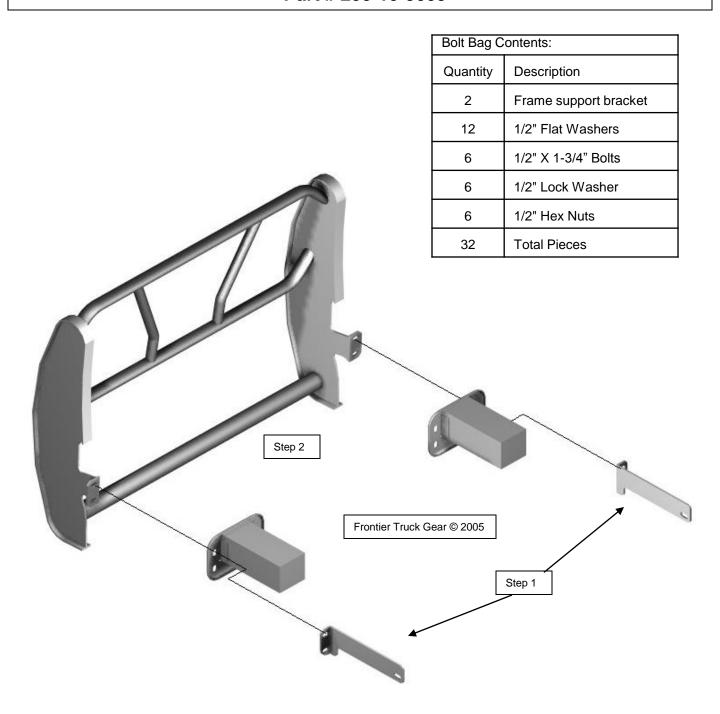
**Step 1:** Install frame support bracket behind frame horn.
