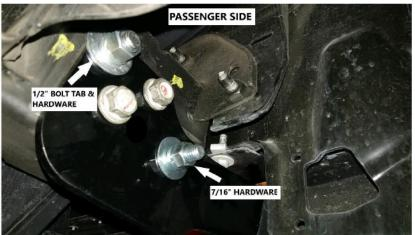
NOTE: It may be easier to install the ½" bolt w/Tab from the hole by the body mount.
