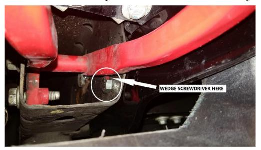
10. Mount the grill guard to the outside of the brackets with the black carriage bolts. Level grill guard and tighten bolts and nuts. You may have to loosen the mounting bracket bolts to help with leveling.
