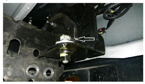
3. (Diesel) On the driver side, cut the front tow hook bolt off. You will use a ½" x 4" bolt to reinstall the tow hook later.
