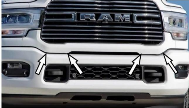
2. If tow hooks are not present, cut out the plastic around the two locations where tow hooks would be *(see photo below)*. If present, remove the factory tow hooks to insert the bottom brackets. **Note: Some trimming to the plastic around the tow hook may be required.**
