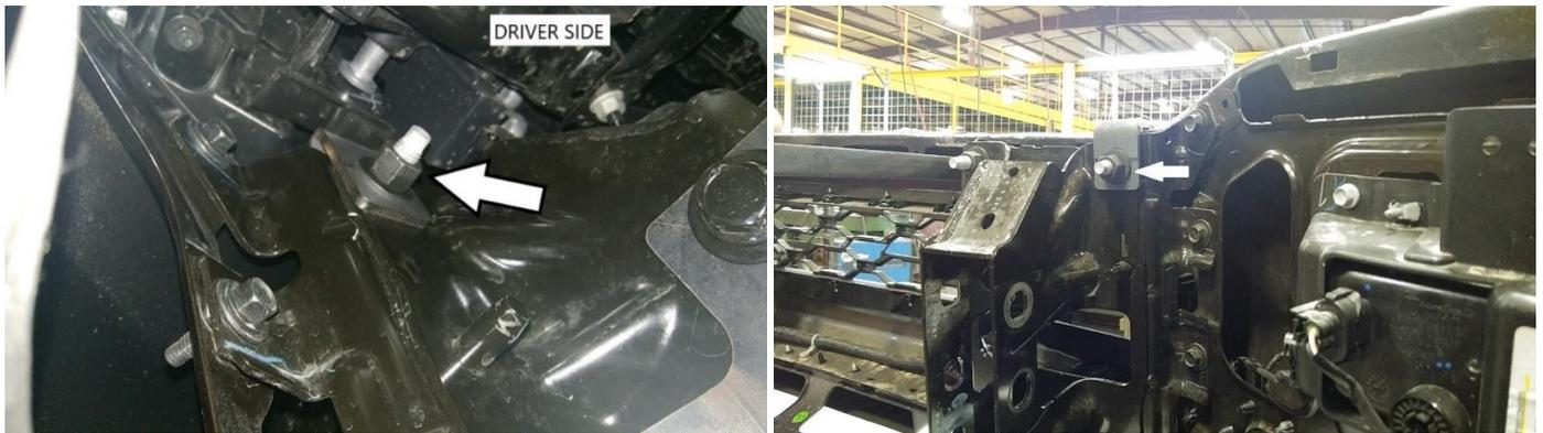
5. Install the grill guard to the bottom brackets. Use black ½" carriage bolts, washers and nuts. Level the grill guard and tighten nuts.
