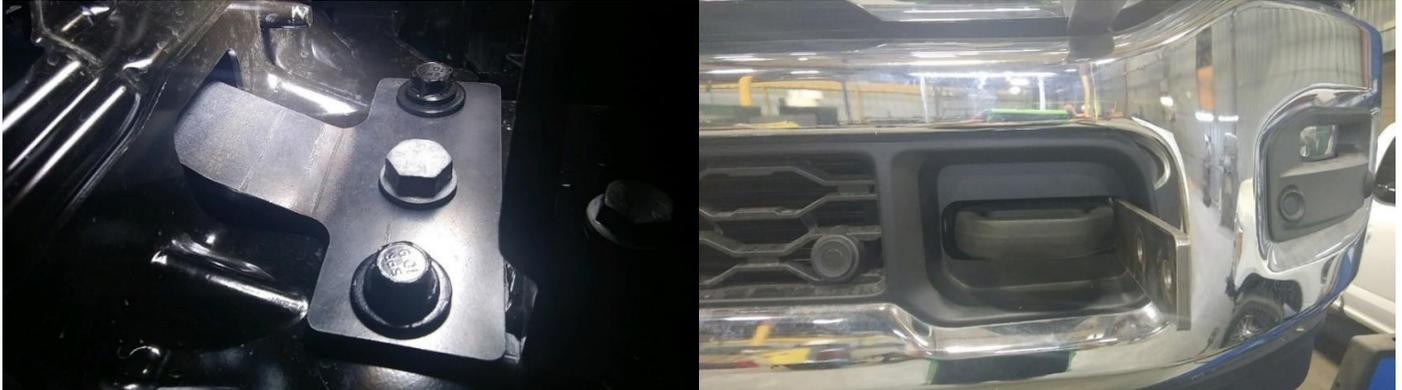
4. Install top mounting bracket. The bracket will be installed from the bottom side of the truck. Remove the top nut of the bumper bracket. Slide the flat side of the top bracket through the opening of the bumper and grille. (1<sup>st</sup> Photo is shown from looking up from under the truck. 2<sup>nd</sup> photo (passenger side) shown with bumper off for location purposes.)
