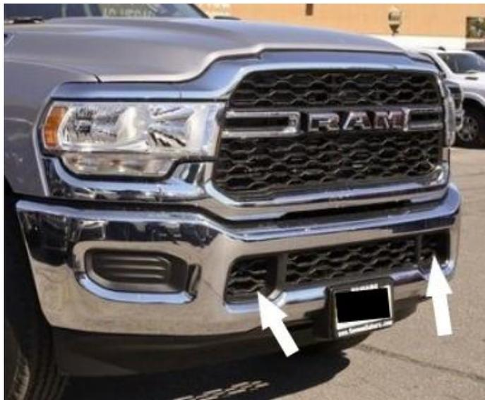
3. Remove the two factory bumper bolts and install the bottom brackets along with tow hooks if present. The brackets will be installed with the bend facing outwards. Note: The bumper bracket will spread out once the bolts are removed. When you try to put the bolts back on, they will seem to be short. If you decide to use the ½" x 4" bolts provided, you will need to drill out the holes in the frame first. *(Photo is of driver side)*
