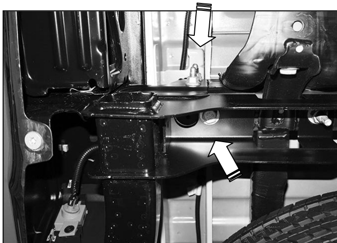
(Fig 3) Remove bumper bolts attaching brackets to frame (arrows). Model with receiver hitch pictured from below
