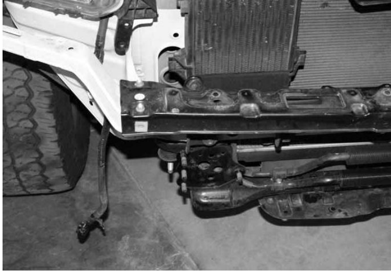
Figure 3 - Factory Bumper Connection
