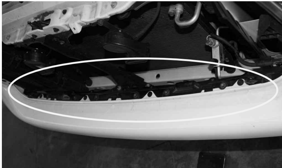
Figure 5 - Center Fascia Fasteners
