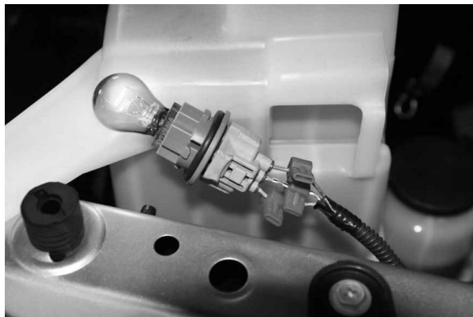
Figure 12 - Turn Signal Wiring Access
