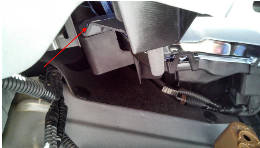
Figure 5 - Pop Clip Location Headlight to Plastic Fascia
