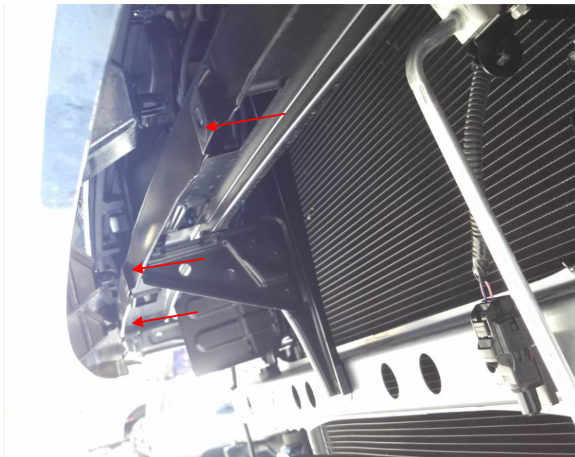
Figure 6 - Grill Plastic Clip Locations
