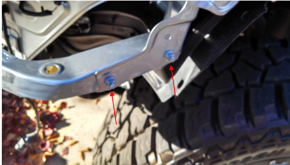
Figure 9 - Fascia Brace Nuts
