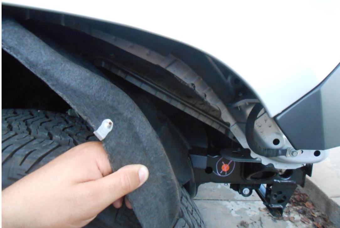
Figure 6a (wheel well liner pull back)
