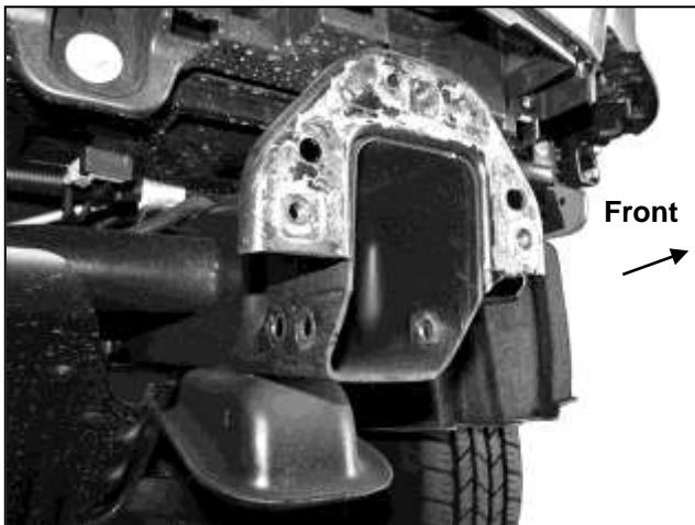
(Fig 5) Remove complete bumper, inner bumper bracket and tow hooks
