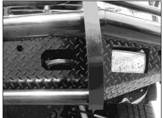
(Fig 16) Reinstall tow hooks with factory hardware
