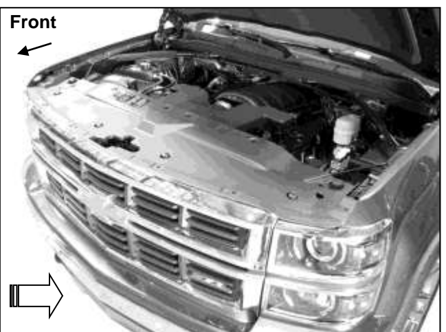
(Fig 2) On 14-15 models, from behind bumper, release clips and hardware attaching plastic fascia panel (arrow) to top of bumper and fender. Remove fascia panel to access grille and bumper hardware from above.
