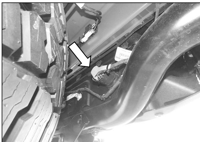
(Fig 1) Unplug the trailer plug, License plate lights and sensors
