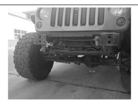
Remove the factory front bumper from vehicle.
