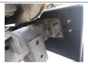
Line up the holes on the frame with the slotted holes on the bumper brackets.
