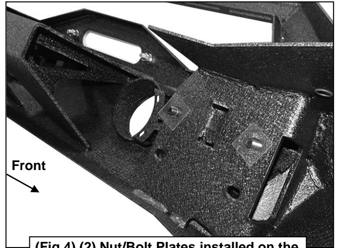
(Fig 4) (2) Nut/Bolt Plates installed on the Passenger/Right back of the Bumper
