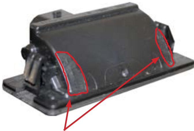
Grind Off The Top Tabs Completely
