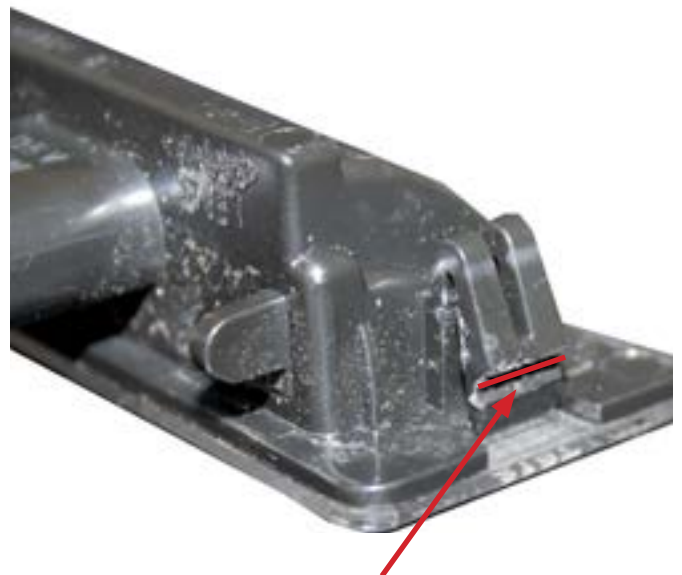
Slightly Trim The Side Tabs Then Test Fit
