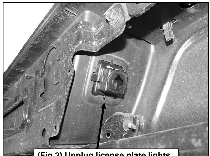
(Fig 2) Unplug license plate lights
