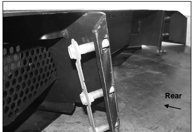
(Fig 4) On models without received hitch, reuse triple bolt plate to attach bumper to ends of frame
