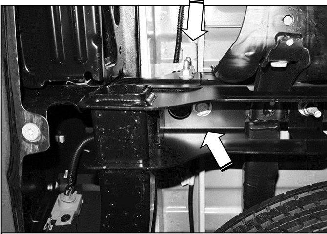
(Fig 3) Remove bumper bolts attaching brackets to frame (arrows). Model with receiver hitch pictured
