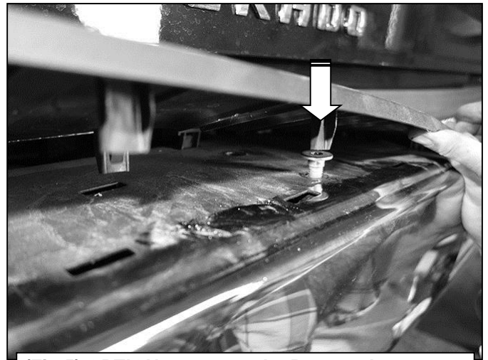
(Fig 5) OPTION 2014-18 only: Remove bumper bolts attaching bumper to inner bracket. Remove outer bumper first, then remove inner brackets
